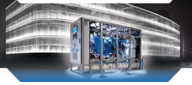
Our ENERGIN® CHP units are compact cogeneration plants with highly efficient heat recovery from the jacket water and the exhaust gas of the gas engine. The innovative design allows an easy and space-saving installation. All major components like gas engine generator unit, heat exchangers, circulation pumps, primary exhaust silencer and control cabinet are factory mounted on a common frame.
